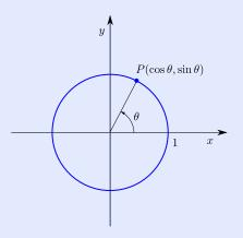
The **cosine** of  $\theta$  (written  $\cos \theta$ ) is defined to be the *x*-coordinate of this point; the **sine** of  $\theta$  (written  $\sin \theta$ ) is defined to be the *y*-coordinate of this point.
