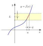
As indicated in the diagram, an altitude band centered at L is determined by specifying a positive number  $\varepsilon$  (epsilon) and similarly, an interval centered at a is determined by specifying a positive number  $\delta$  (delta). So, the condition can be expressed succinctly by saying: Given any positive number  $\varepsilon$ , there exists a positive number  $\delta$  that "works."
